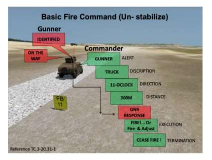
Figure 1. Example of basic fire command sequence for an unstabilized gunnery platform.
