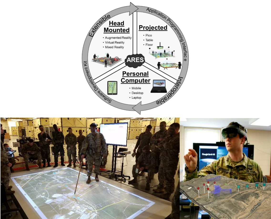
Figure 1. Augmented Reality Sand Table (Ares) visualization modalities, with floor projection and augmented reality examples.
